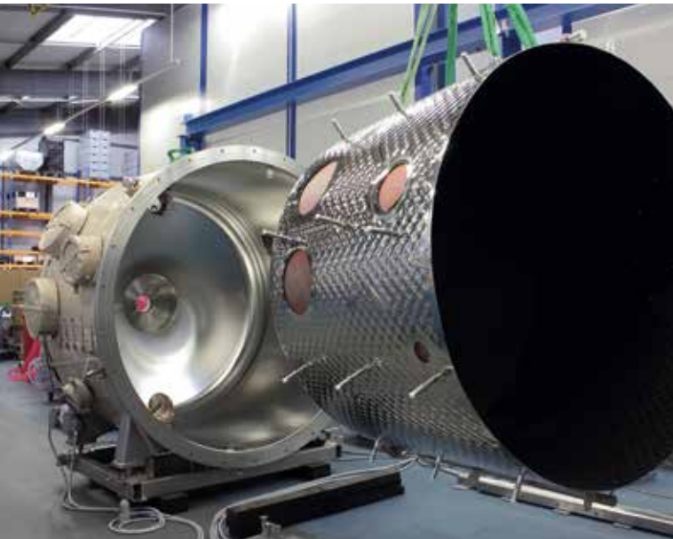
The space simulation chamber for the CHEOPS mission. The chamber is shrouded with a clean-room-compatible insulation
